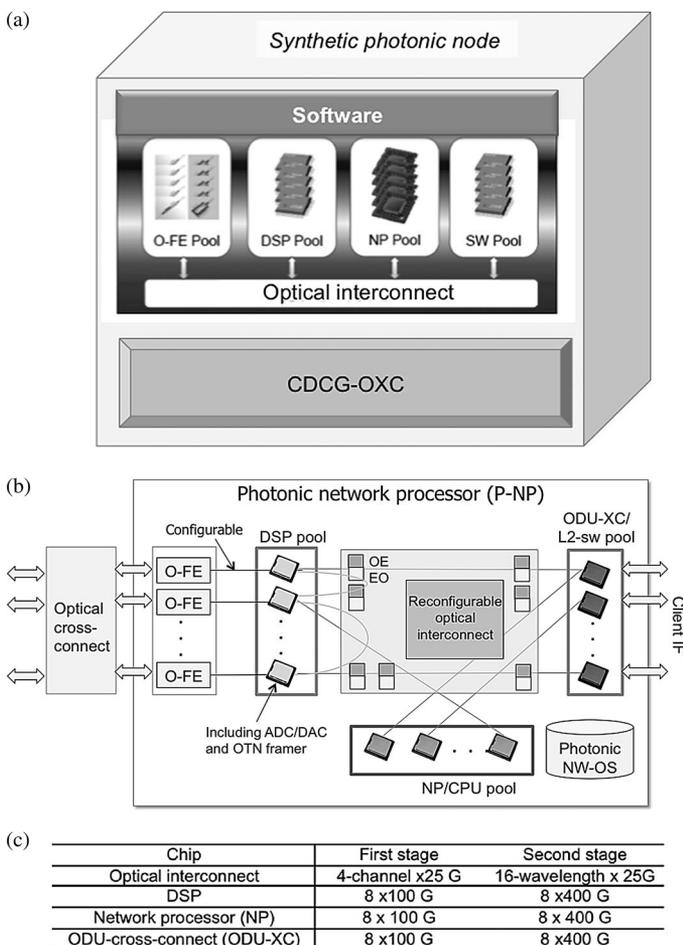
Fig. 6. (a) Architecture of a synthetic photonic node, (b) photonic network processor (P-NP) consisting of pools of DSPs, NPs, and ODU-XCs/L2-SWs, connected with reconfigurable optical interconnect, and (c) projected stages of the optical interconnect.
