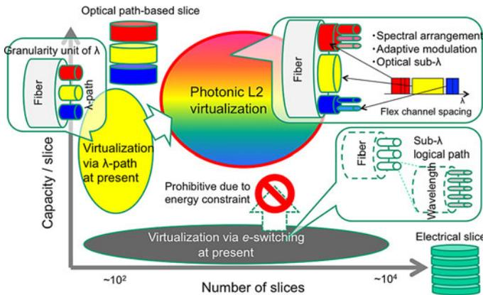
Fig. 3. Capacity per slice as a function of the number of slices for conventional virtualization using electrical and wavelength paths. Photonic layer 2 (P-L2) virtualization fills the vacancy of conventional virtualization techniques.
