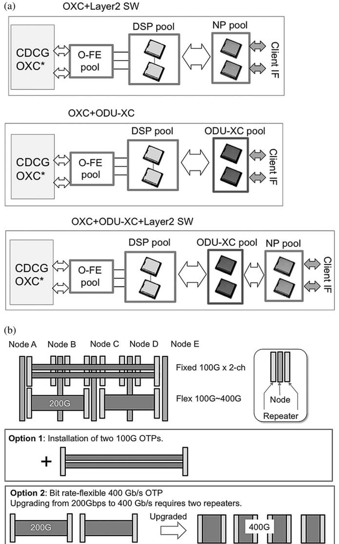
Fig. 8. (a) Use case 1: Multi-functional CDCG-OXC; with layer 2 switch, ODU-XC, and ODU-XC and layer 2 switch. (b) Use case 2: Upgrading scenarios of optical transponder (OTP): conventional bit rate-fixed OTP vs. bit rate-flexible OTP.
