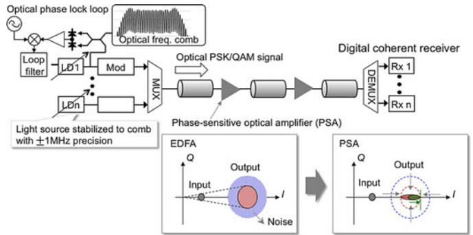
Fig. 2. In-line phase-sensitive amplifier (PSA) in a trunk line along with a frequency-stabilized optical transmitter using optical phase lock loop.
