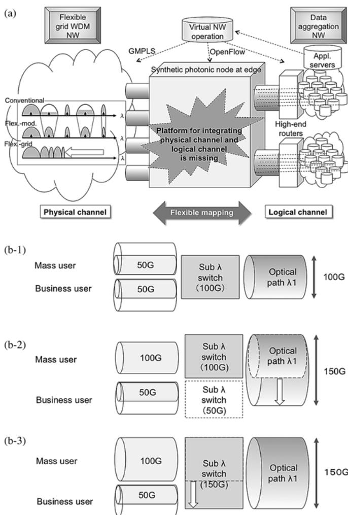
Fig. 5. (a) Contrast between the logical channel of an IP network and the physical channel of a flexible grid WDM transport network where the bridging functionality of flexible mapping technology is currently missing, and (b) upgrade scenario of a sub-wavelength switch when demand arises for another 50 G bandwidth from mass users.
