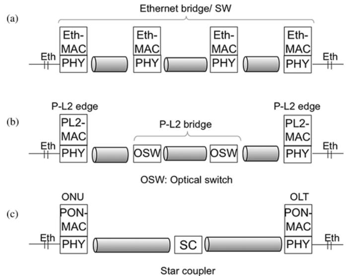
Fig. 4. Comparison of network architecture. (a) Multi-hop Ethernet switch network, (b) photonic layer 2 (P-L2) network, and (c) Ethernet passive optical network (PON).
