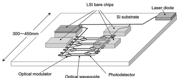
Fig. 7. Conceptual schematic of silicon optical interposer integrated with LSI bare chips. A laser diode, arrays of eight optical modulators and eight photodetectors are integrated on a silicon substrate. LSI bare chips are mounted on the interposer, and are electrically connected to the optical modulators and photodetectors.
