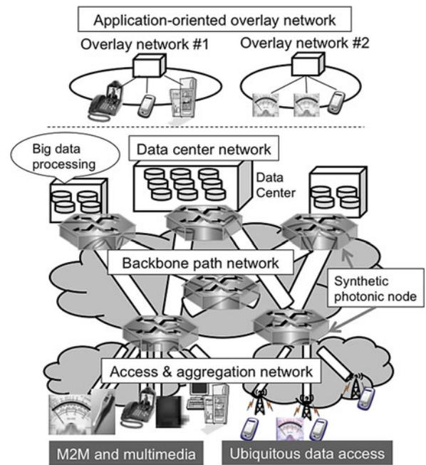
Fig. 1. Conceptual schematic of the Smart Photonic Cloud (SPC) for the Big Data era in 2020. A backbone path network consisting of synthetic photonic nodes that interconnects data center networks and access and aggregation networks with flexible optical L1/L2 paths. Various application-oriented overlaid networks are created on it.
