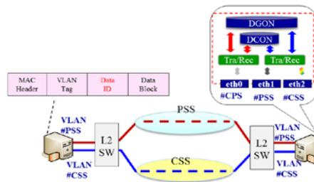
Figure.10. Communication between Two Nodes of DCON
