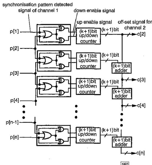
Fig. 1 Proposed circuit for counting offset clock cycles
