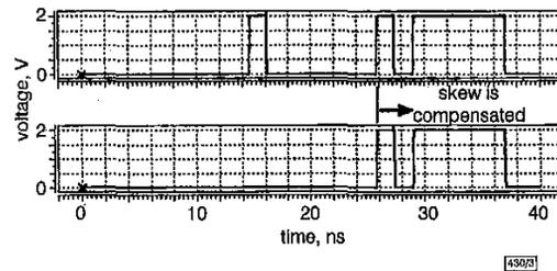
Fig. 3 Simulated skew-compensated output signals
