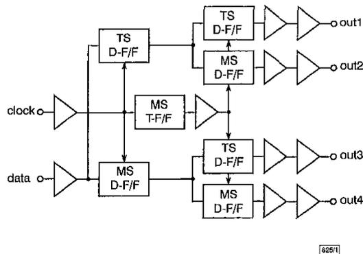
Fig. 1 Block diagram of 1:4 demultiplexer IC
