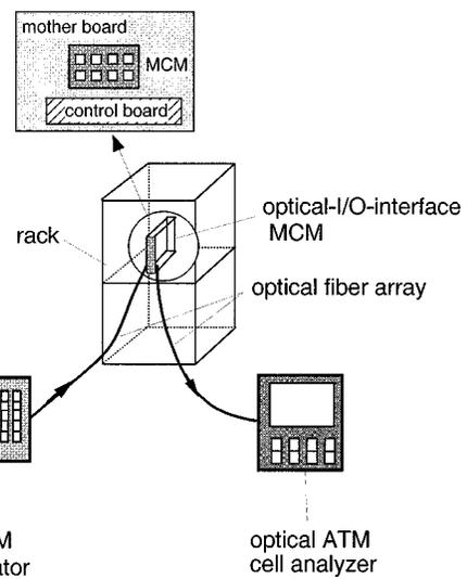
Fig. 12. System for evaluating optical I/O MCM.
