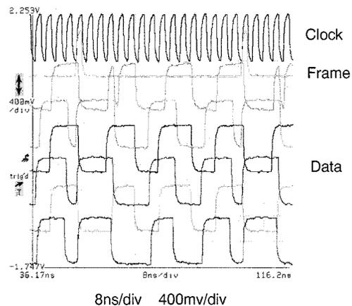
Fig. 13. Operating waveforms of optical I/O MCM (at 625 Mb/s).
