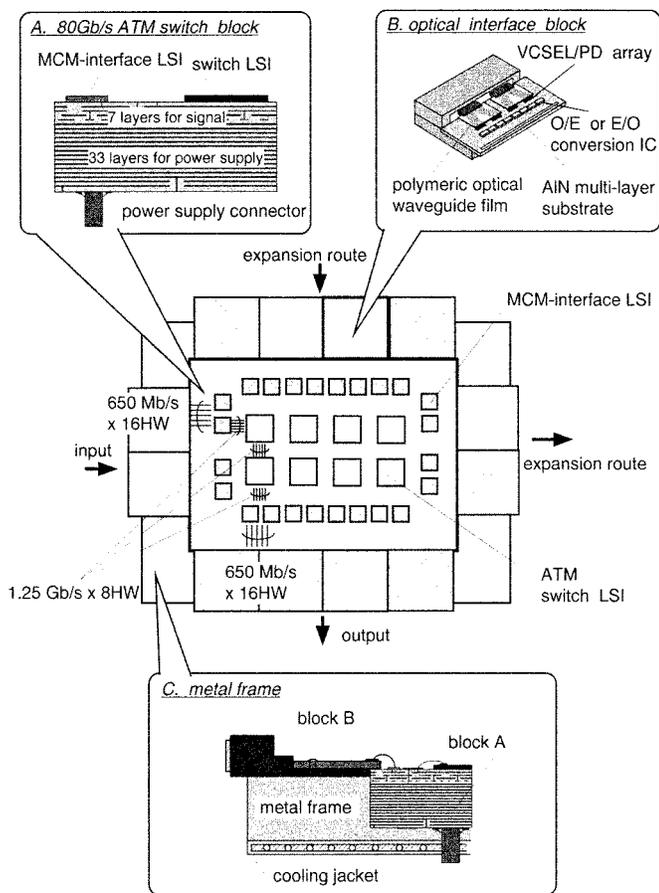
Fig. 3. Structure of the optical I/O interface MCM.
