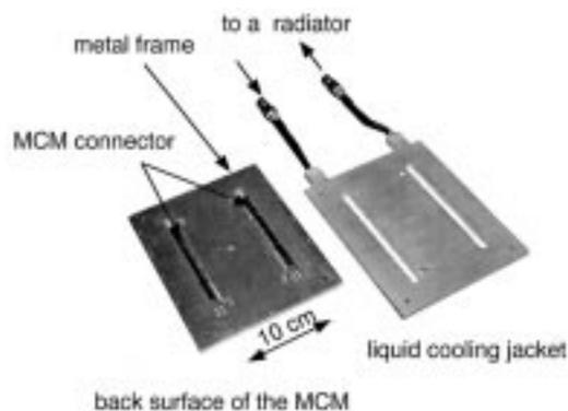
Fig. 4. Photograph of the liquid cooling jacket.
