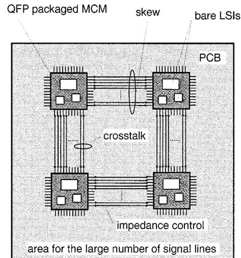
Fig. 1. Conventional module-to-module interconnection.
