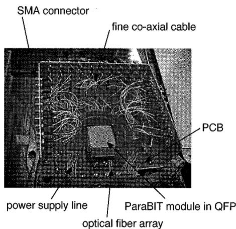
Fig. 11. E/O converter for system evaluation.
