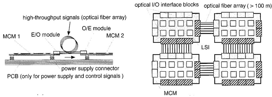
Fig. 2. Concept of the optical I/O interface MCM.
