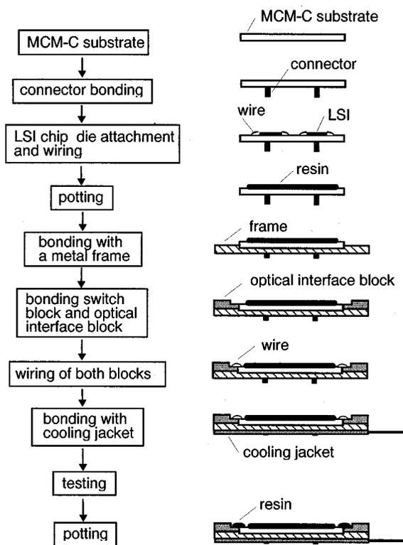
Fig. 5. Fabrication process of the module.
