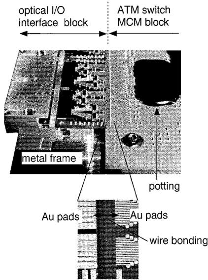
Fig. 6. Au wire-bonding pad configuration of each block.
