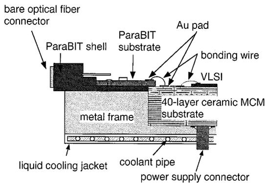
Fig. 7. Details of connections in each block.
