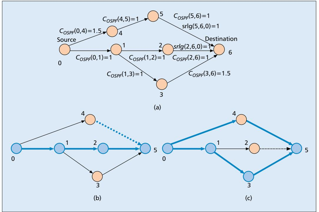
■ **Figure 2.** Disjoint path selection with SRLG constraints: a) network example; b) conventional algorithm; c) WSRLG algorithm.
