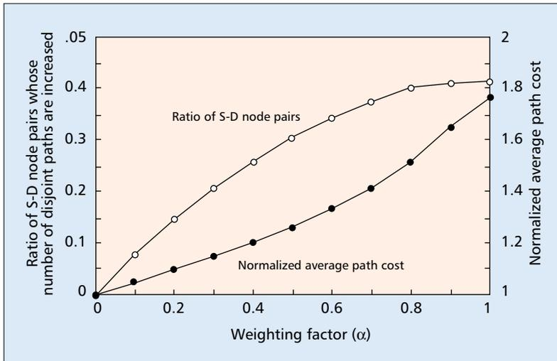
■ **Figure 3.**  $\alpha$  vs. ratio of S-D node pairs whose number of disjoint paths is increased and path cost  $D_{path}(s, d)$ . ( $N = 20$ ,  $D = 6$ ,  $G = 16$ ,  $m = 14$ .)
