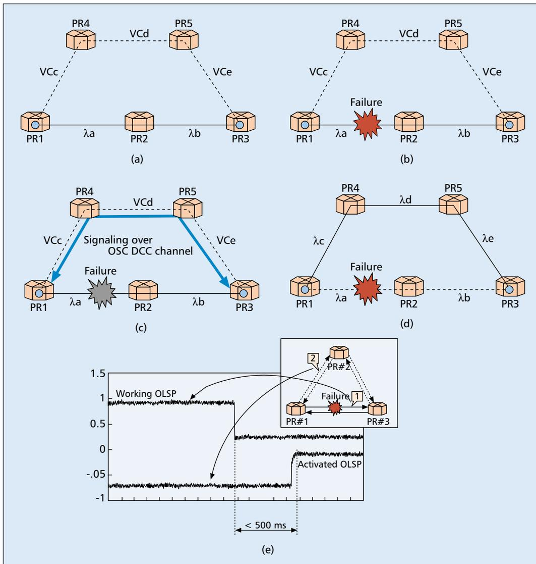
■ **Figure 4.** Fast restoration procedure: a) restoration configuration; b) link failure; c) signaling for restoration path configuration; d) restoration completion; e) experimental results of restoration demonstration. PR: photonic MPLS router, VCx: virtual channel on DCN;  $\lambda_x$ : OLSP with wavelength  $x$ .
