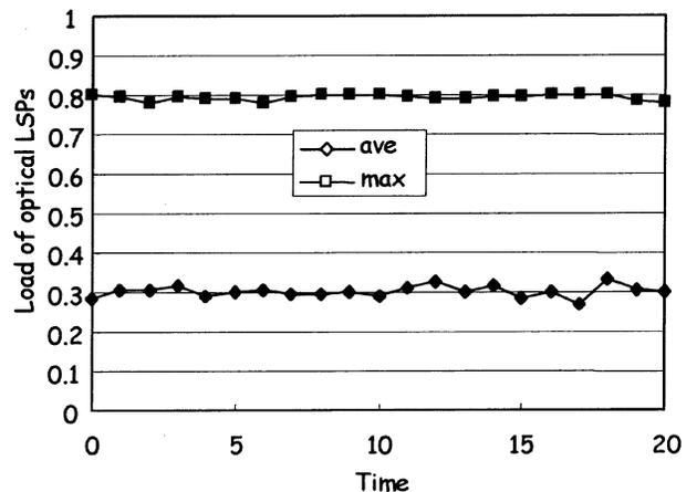
Fig. 15. Load of optical LSPs as a function of time sequence:  $(r_0, r_1) = (0.1, 0.2)$ .
