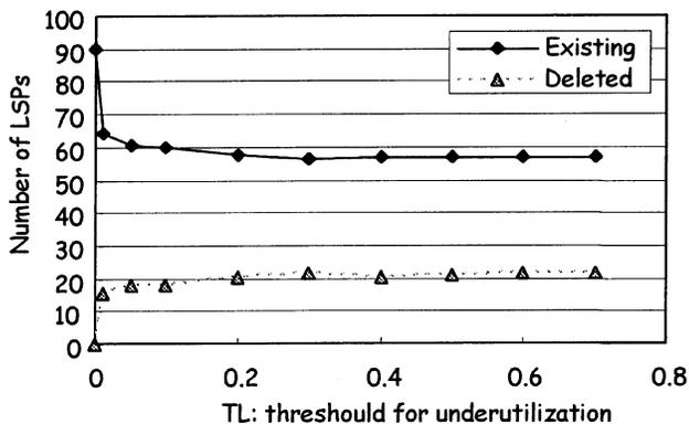
Fig. 18. Relationship between the threshold for underutilization and the number of optical LSPs.
