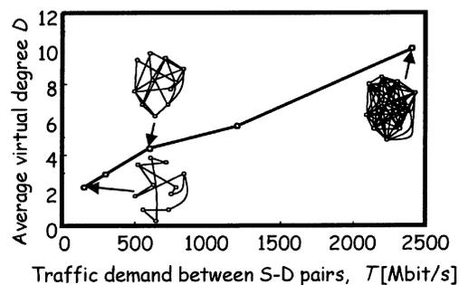
Fig. 9. Average virtual degree as a function of traffic demands backed up by wavelength.
