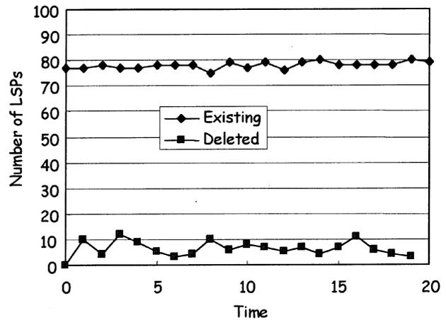
Fig. 13. Number of lightpaths as a function of time sequence:  $(r_0, r_1) = (0.125, 0.175)$ .
