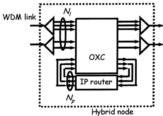
Fig. 1. Hybrid node architecture (unfolded view).
