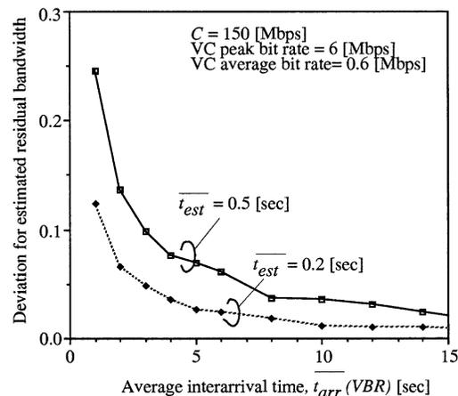
Fig. 8 Accuracy of estimated residual bandwidth.
