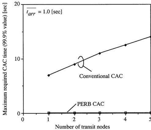
Fig. 4 Response time in CAC systems for multiple nodes.
