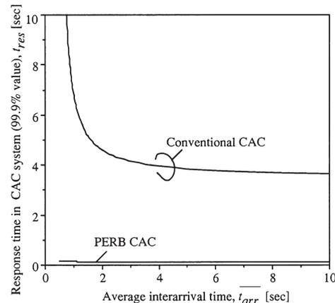
Fig. 3 Response time in CAC systems for single node.
