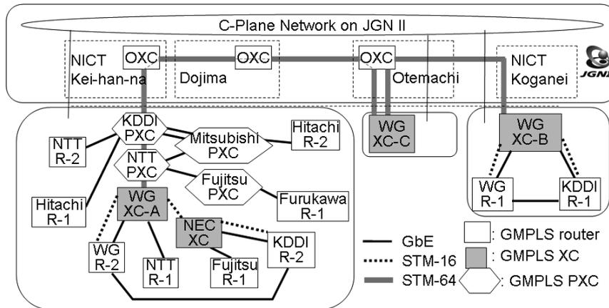
Fig. 3 GMPLS multi-vendor multi-layer interoperability field trial test setup in the Kei-han-na Open Laboratory.
