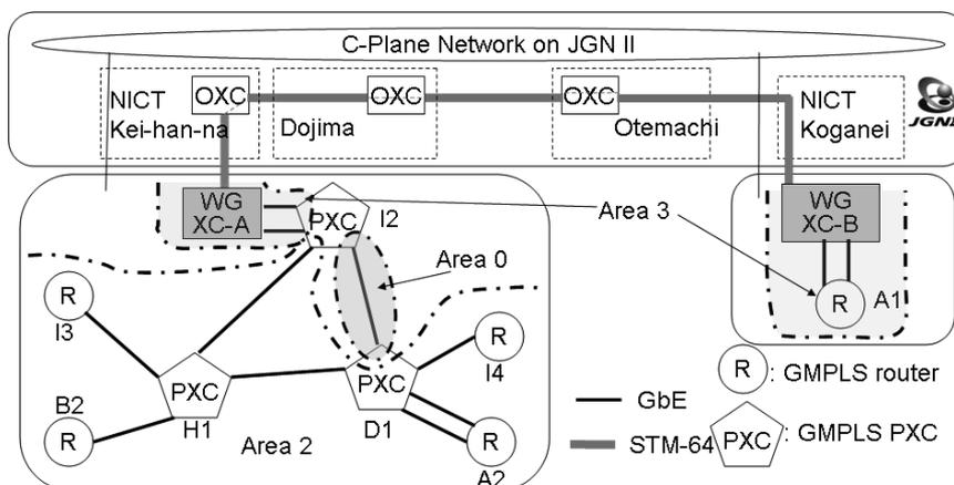
Fig. 6 GMPLS multi-vendor multi-OSPF domain interoperability field trial test setup in the Kei-han-na Open Laboratory.
