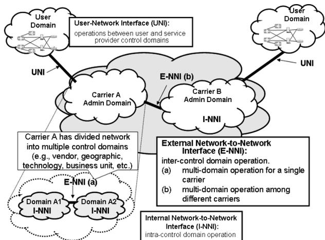
Fig. 2 Reference model of multi-carrier networks.
